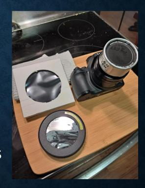
• I've settled on solar filter film sandwiched between two cheap camera filters on a flip up filter holder.
