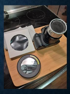
I've settled on solar filter film sandwiched between two cheap camera filters on a flip up filter holder.
